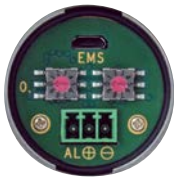
Thermalert 4.0 supports 2-wire loop
